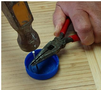
Use the hammer, nail and pliers to put 6 to 10 holes in the lid. Pliers help hold the nail safely.
