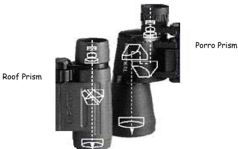
The two most frequently used prism systems are porro and roof. **Porro Prism** binoculars are characterized by the eyepieces being offset from the objective lenses. These also tend to be bulkier but less expensive. **Roof Prism** binoculars feature lenses positioned in line providing for a more compact design but are usually more expensive than porro prism binoculars.
